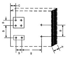
Scheme of edge distance and spacing in thin-wall concrete elements
