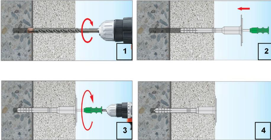
1) Drill the hole perpendicular to the substrate surface. Clean the drill hole.
