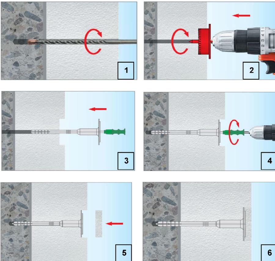
1) Drill the hole perpendicular to the substrate surface. Clean the drill hole.
